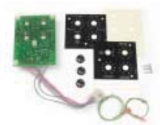
Optional time controls for pre-flow and post-flow gas, burnback, as well as cold inch and gas purge control.
